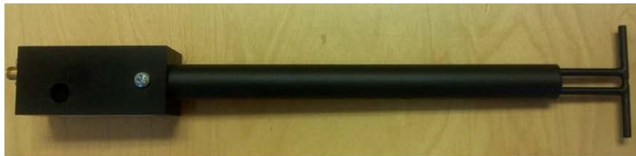
Figure 1 – MVG COMOSAR Validation Dipole
