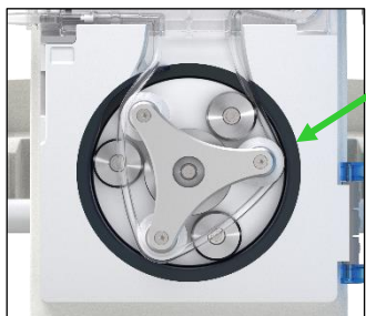
Figure 51. Position of the white guide roller to 2–3 o'clock
