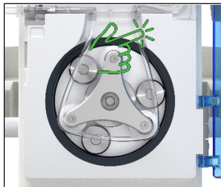
Figure 50. Pressing in the tubing segment
