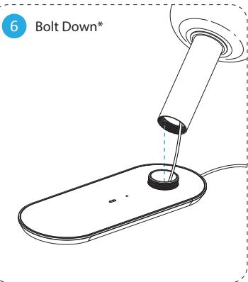
[\*Optional step] To bolt down the Combi onto a tabletop, slowly unscrew the vertical stem from the body.
