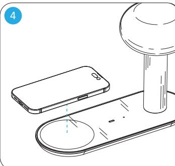
Place any smart device that supports the Qi wireless charging standard onto the ring to charge wirelessly.
