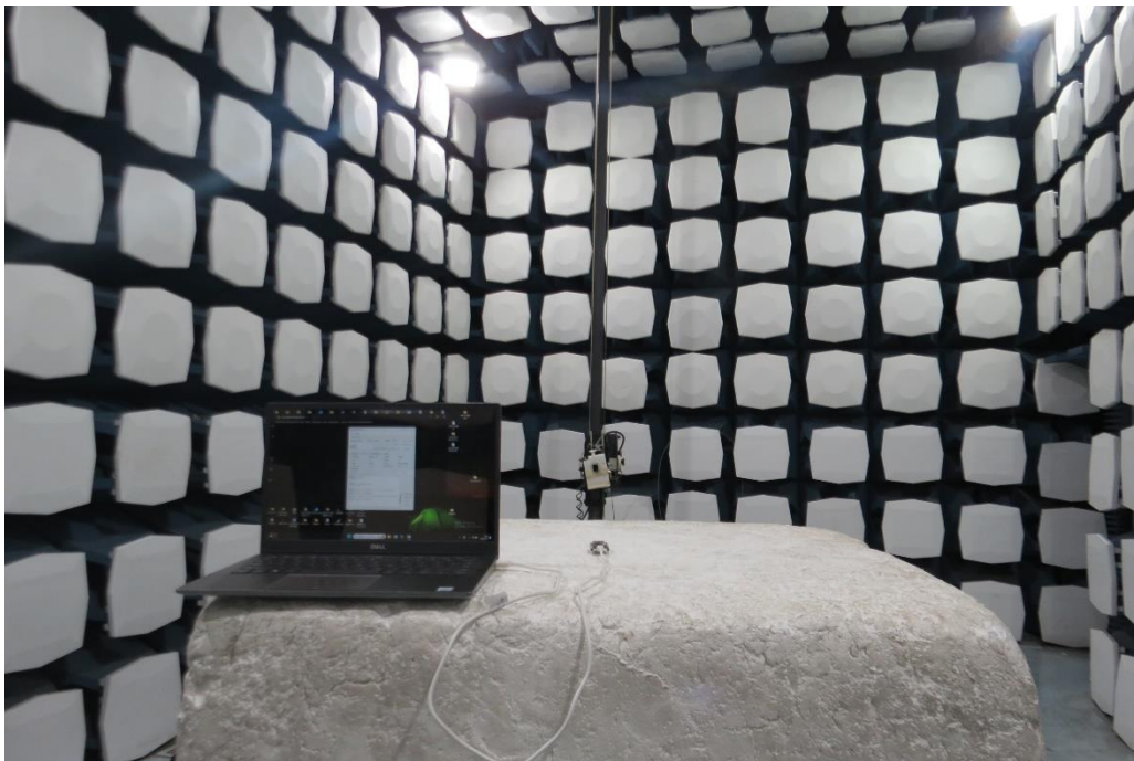
Picture 1 Radiated Emission Test Setup
