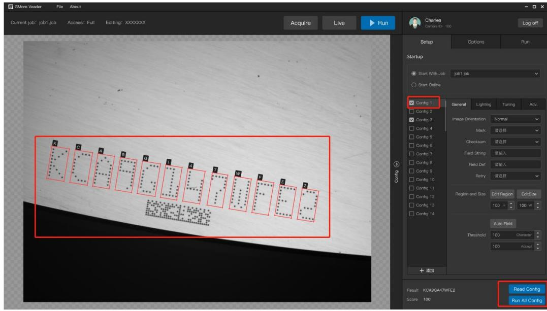
After the configuration setting is completed, check multiple configurations in the configuration list and click **Run All Config**, then the system conducts image reasoning with all the current configurations to show the identification effect, and go to the **Run** table. You can click to switch the corresponding identification result of each **config** configuration.
