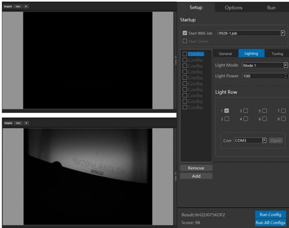
**Note: Imaging Orientation** setting to ensure that the imaging is frontal imaging. If the image is 180° angle as shown below, set the **Image Orientation** to **Rotated 180 Degree** to fix it.
