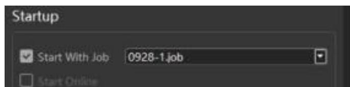
After **Start With Job** checkbox is enabled, the configuration of the current job is available during runtime operation.
