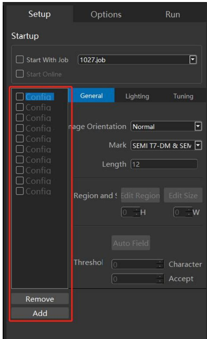
Each file job supports multiple configurations for different wafer surfaces. When multiple configurations are set, the highest score is sent to the console for the current wafer after each read.
