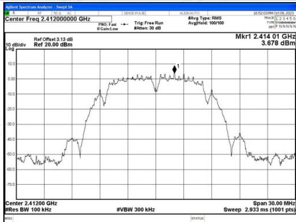
Band Edge NVNT b 2412MHz Ant1 Emission
