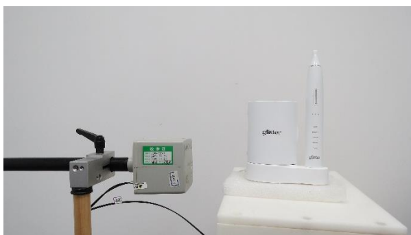
Picture 4: Left Edge, the distance from EUT to the bottom of the Phantom is 20cm
