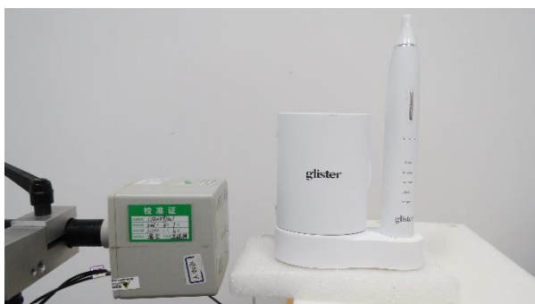
Picture 9: Left Edge, the distance from EUT to the bottom of the Phantom is 15cm
