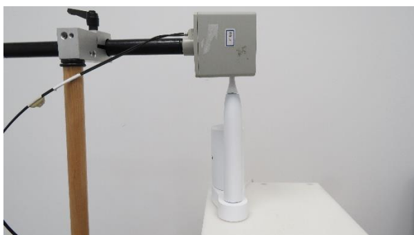
Picture 16: Top Edge, the distance from EUT to the bottom of the Phantom is 0cm
