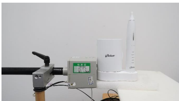
Picture 14: Left Edge, the distance from EUT to the bottom of the Phantom is 0cm
