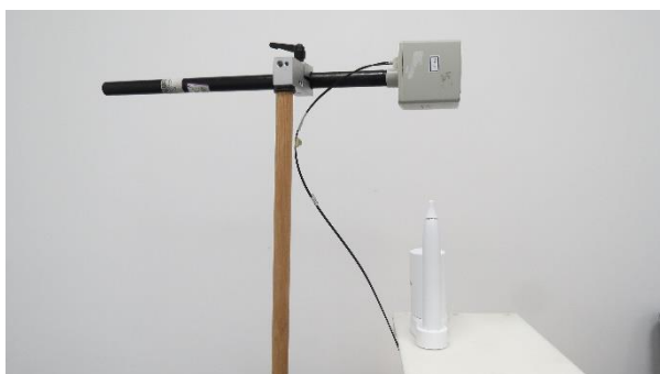
Picture 6: Top Edge, the distance from EUT to the bottom of the Phantom is 20cm
