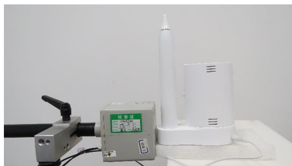
Picture 15: Right Edge, the distance from EUT to the bottom of the Phantom is 0cm
