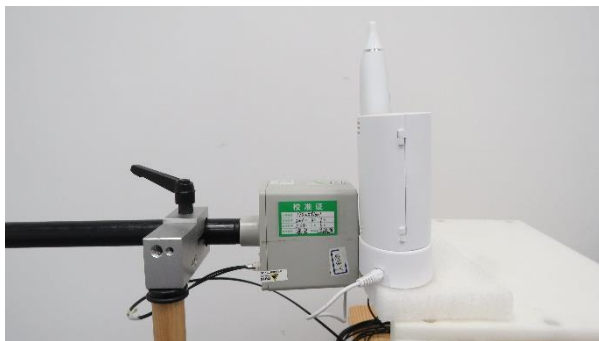
Picture 12: Back Side, the distance from EUT to the bottom of the Phantom is 0cm
