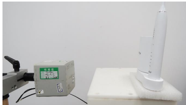
Picture 3: Front Side, the distance from EUT to the bottom of the Phantom is 20cm
