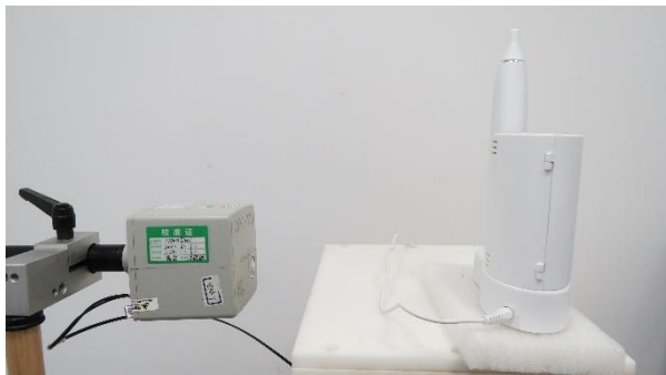
Picture 2: Back Side, the distance from EUT to the bottom of the Phantom is 20cm
