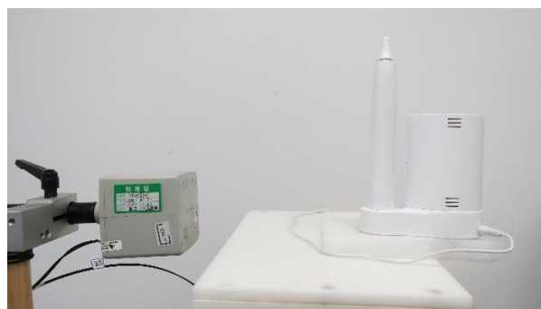
Picture 5: Right Edge, the distance from EUT to the bottom of the Phantom is 20cm
