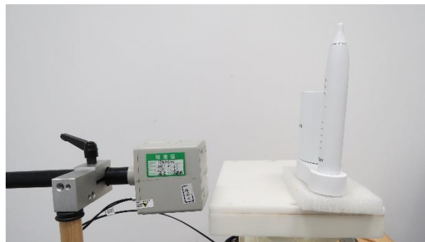
Picture 8: Front Side, the distance from EUT to the bottom of the Phantom is 15cm
