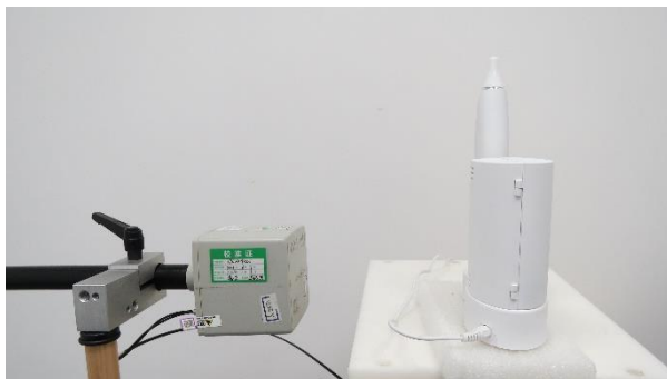
Picture 7: Back Side, the distance from EUT to the bottom of the Phantom is 15cm
