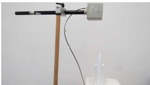
Picture 11: Top Edge, the distance from EUT to the bottom of the Phantom is 15cm
