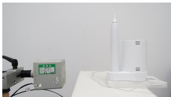
Picture 10: Right Edge, the distance from EUT to the bottom of the Phantom is 15cm
