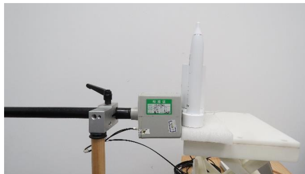
Picture 13: Front Side, the distance from EUT to the bottom of the Phantom is 0cm
