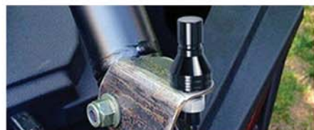
Step 4: Tighten aluminum base in the hole
