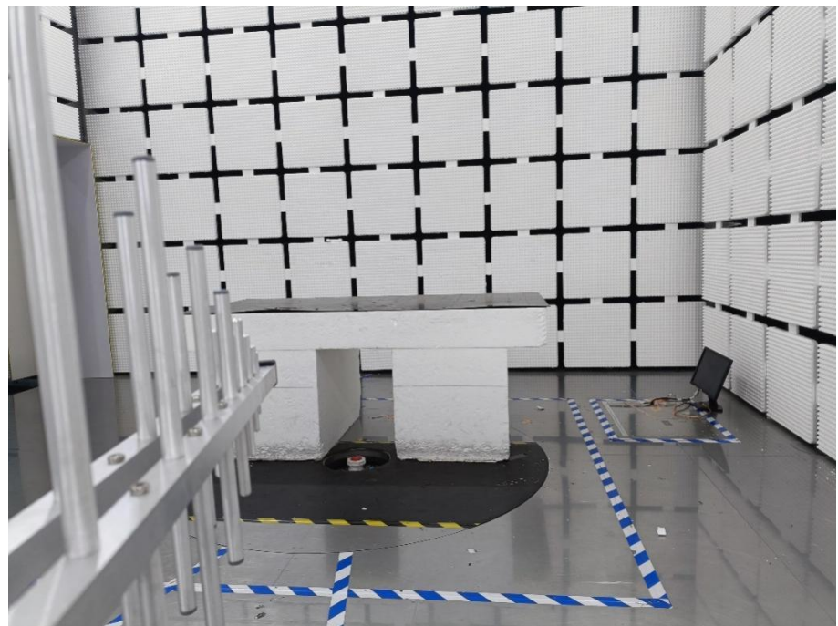
Radiation Emission Test Setup (30MHz to 1GHz)
