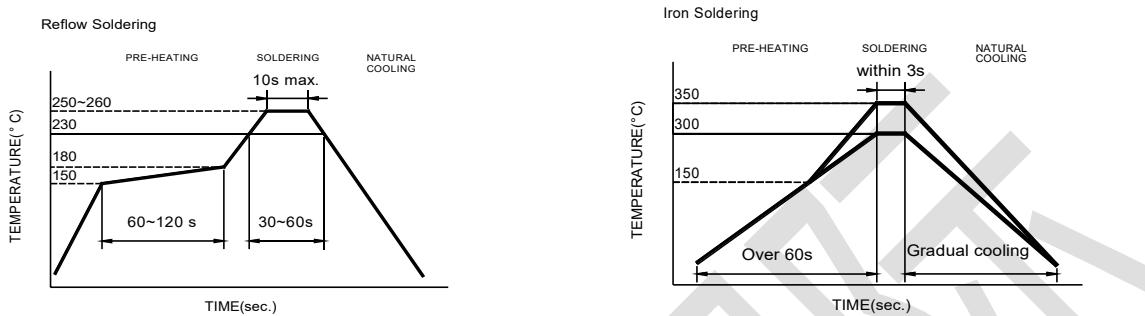
Recommended temperature profiles for re-flow soldering in Figure 1.
