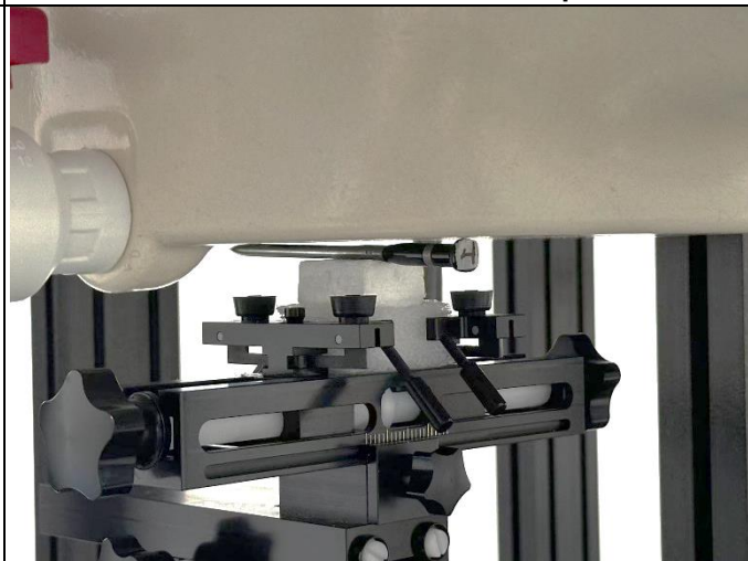
Side 4 of EUT + Probe with 0 cm Gap
