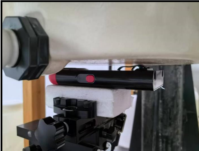
Rear Face of EUT with 10 mm Gap
