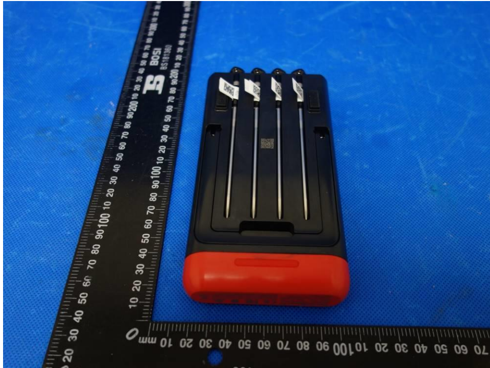
Figure 3: Overview (Device Base and Probe of model WT06)
