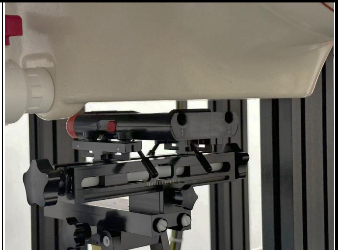
Rear Face of EUT with 10 mm Gap
