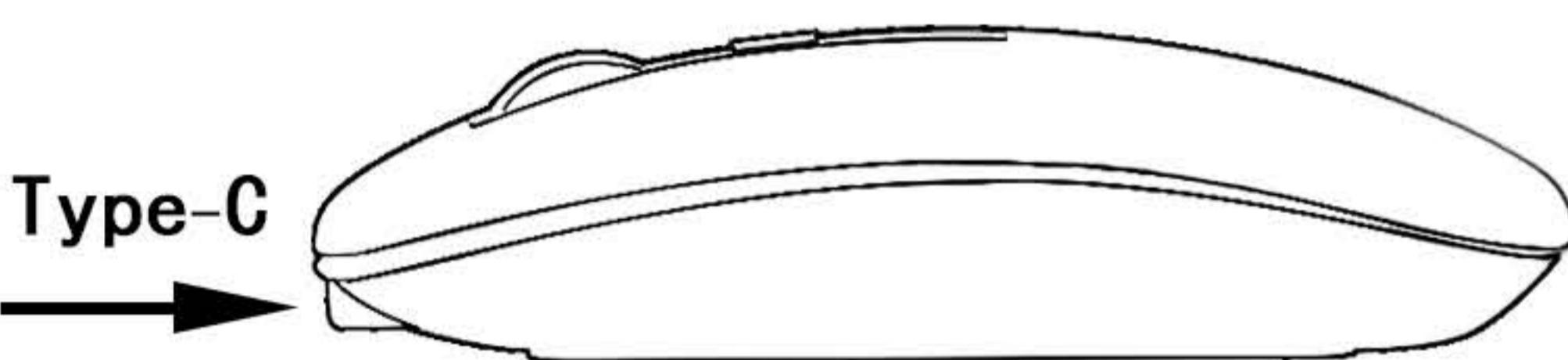
Charging cable connected to the computer is USB, charging when the red light, the charging process is about 1-2 hours, charging complete the red light goes off
