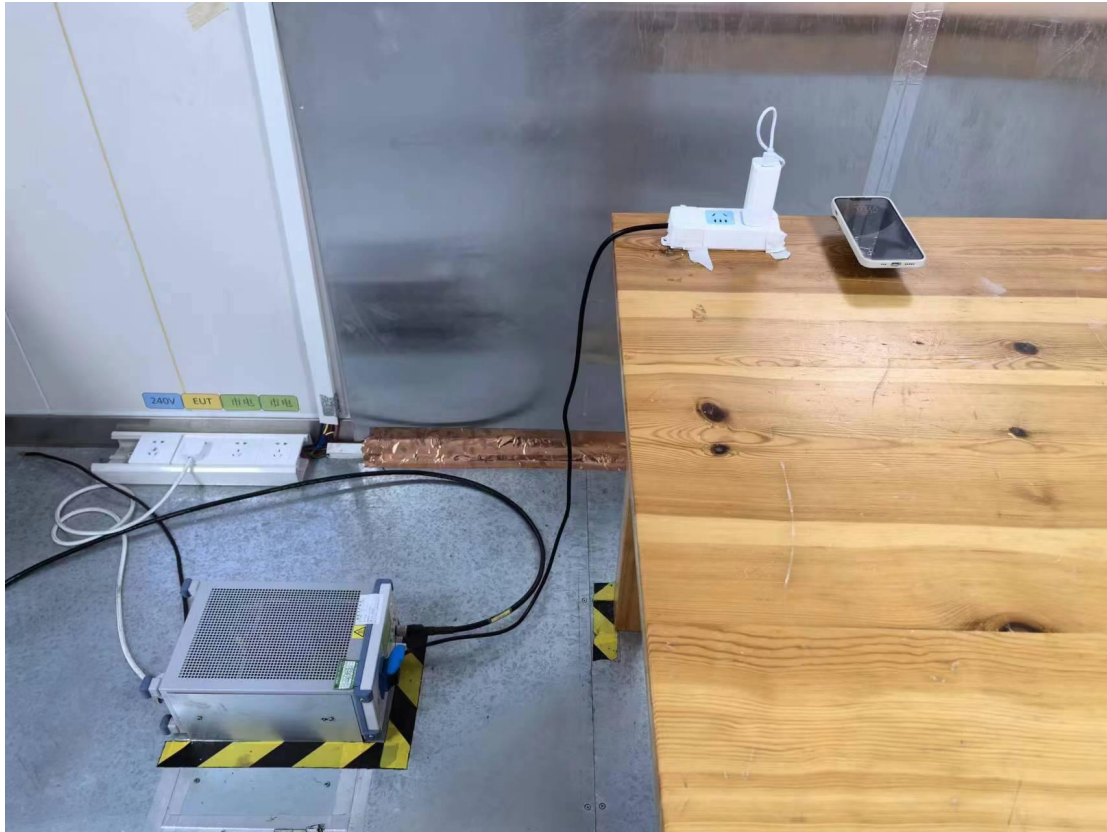
Conducted emission test setup
