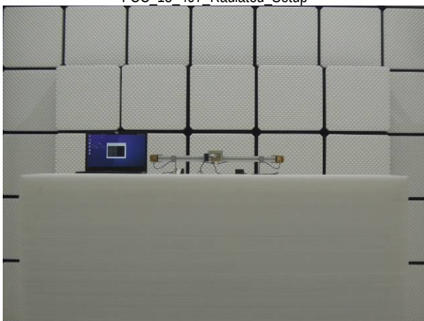
FCC 15 407 Radiated Setup
