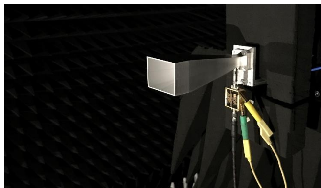
Fig. 3 Test horn antenna DRH1067 with connected amplifier.
