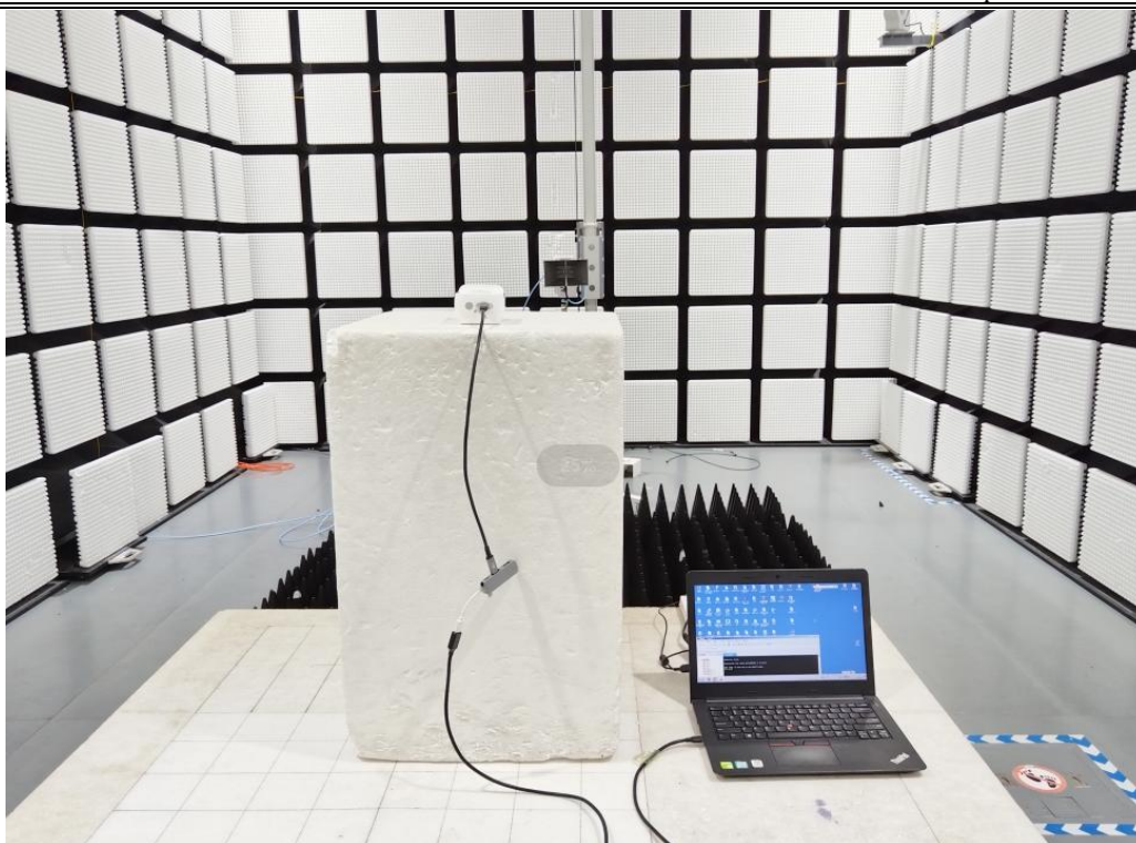
Fig. 3 Radiated emission setup photo(Above 1GHz)
