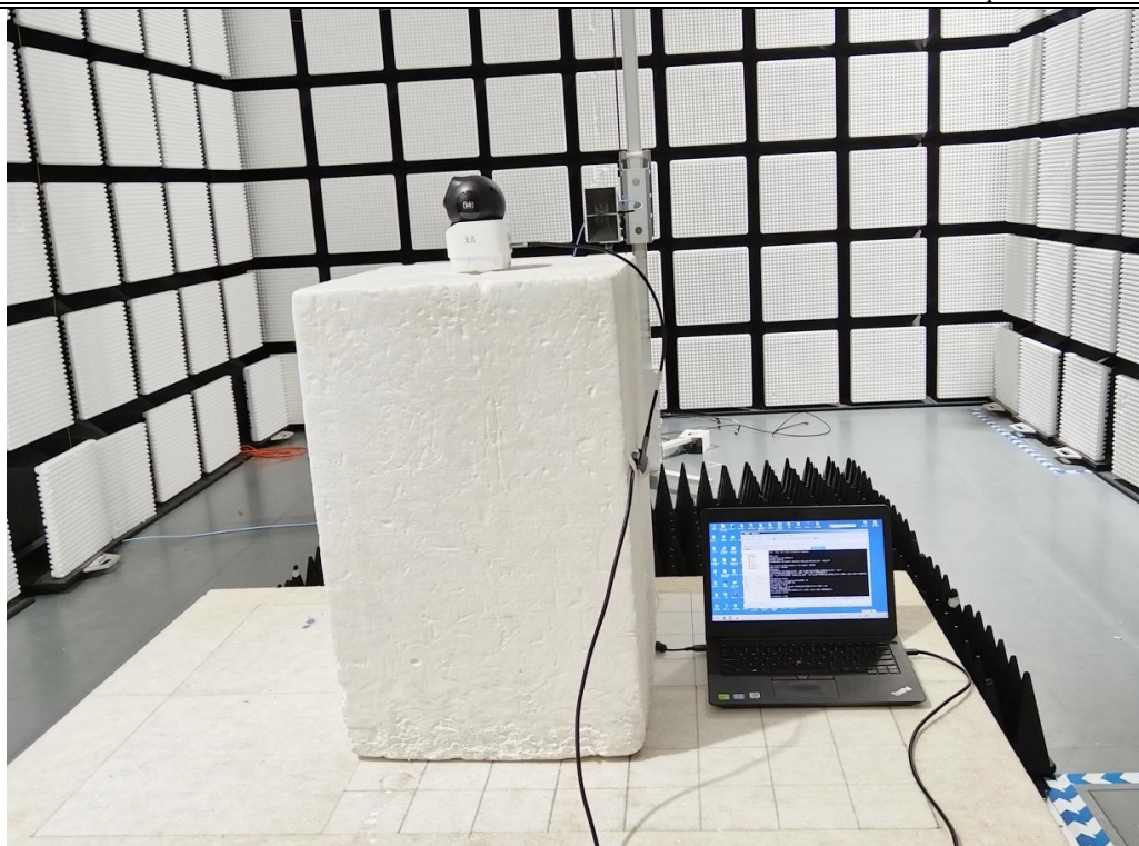
Fig. 3 Radiated emission setup photo(Above 1GHz)
