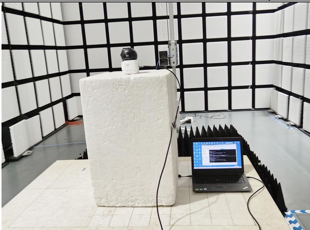
Fig. 3 Radiated emission setup photo(Above 1GHz)
