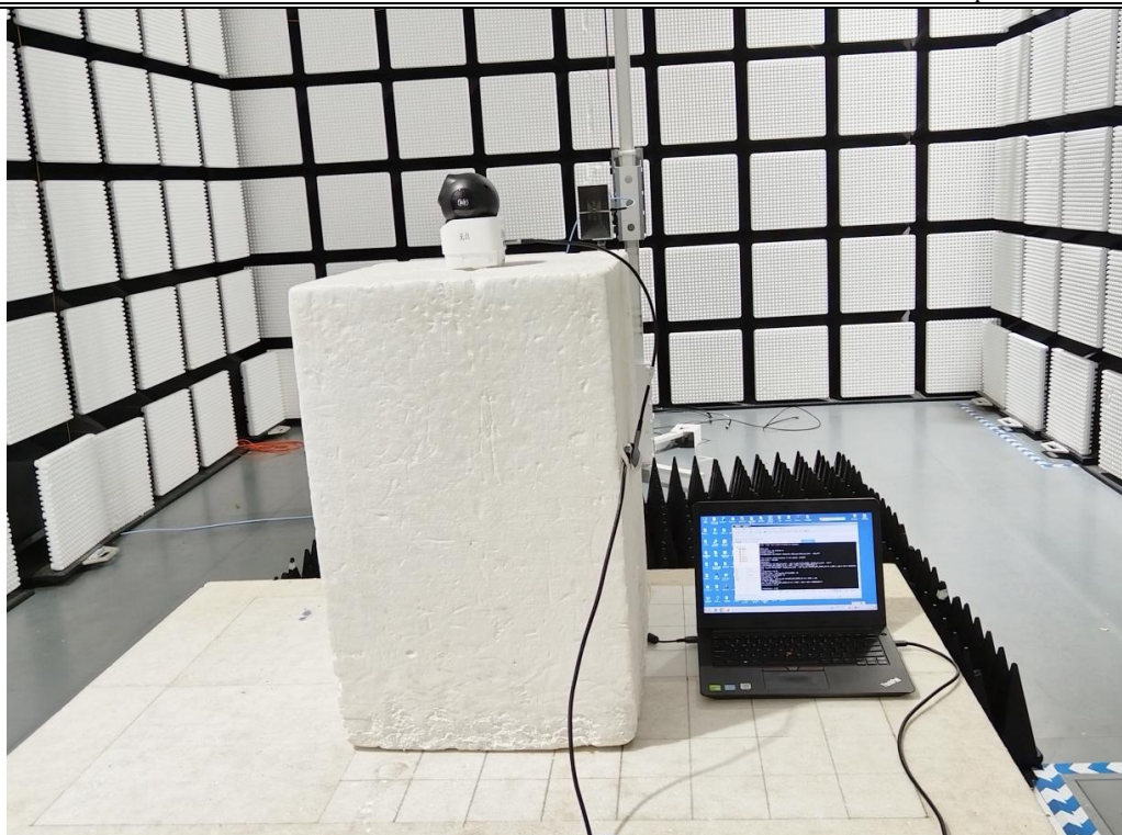
Fig. 3 Radiated emission setup photo(Above 1GHz)
