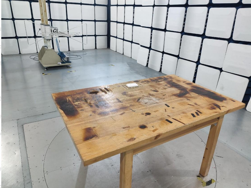
Photo of Radiation Emission Test (below 1GHz)
