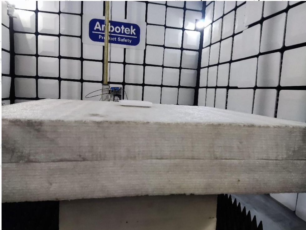
Photo of Radiation Emission Test (above 1GHz)
