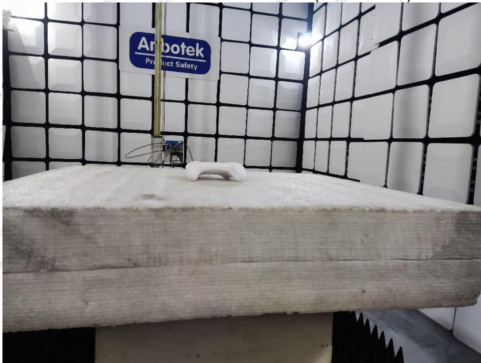
Photo of Radiation Emission Test (above 1GHz)
