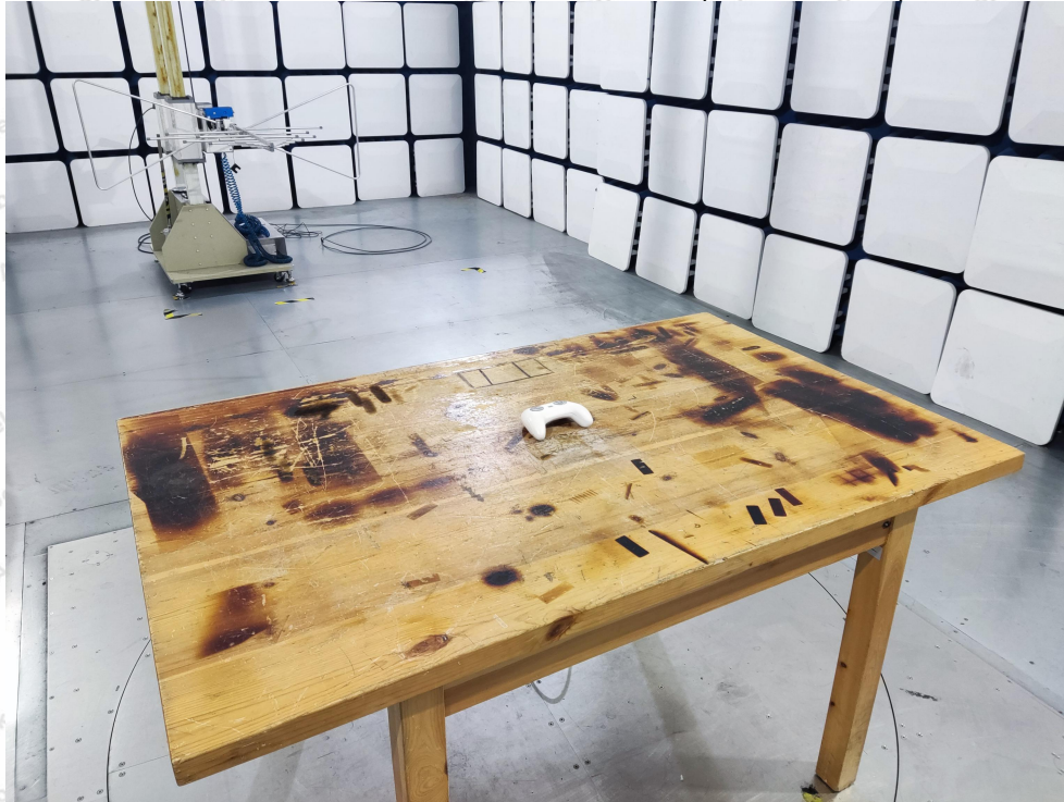
Photo of Radiation Emission Test (below 1GHz)
