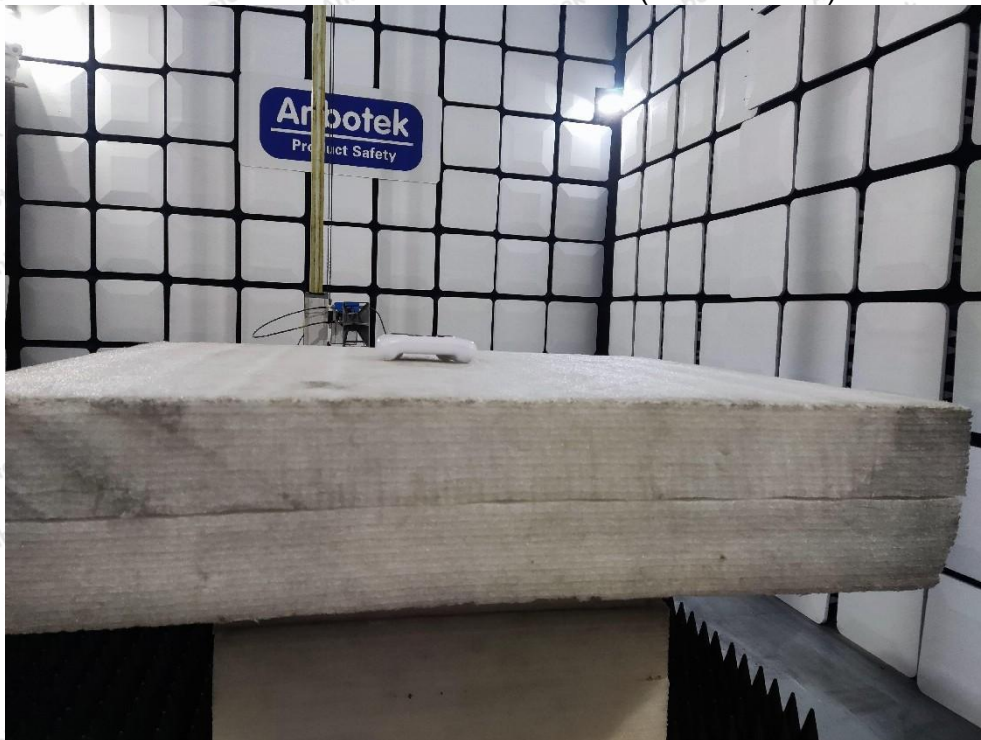
Photo of Radiation Emission Test (above 1GHz)
