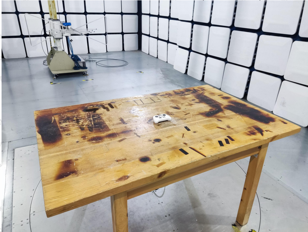
Photo of Radiation Emission Test (below 1GHz)
