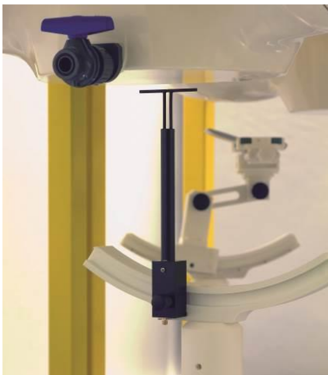
Setup Photo of Dipole Antenna
