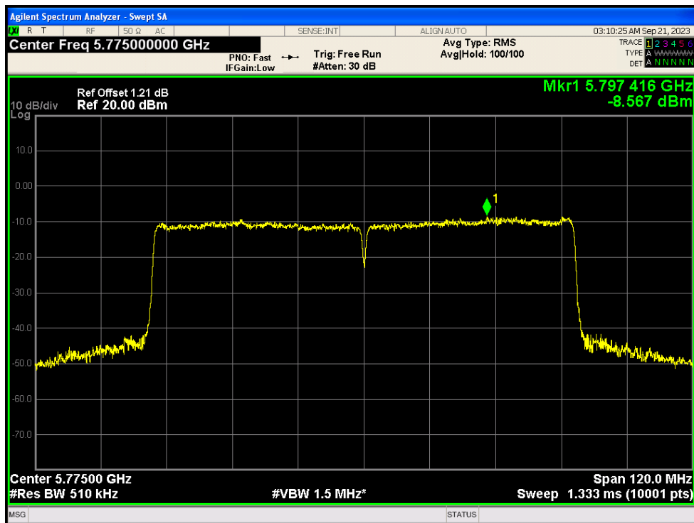
PSD NVNT ac80 5775MHz Ant2
