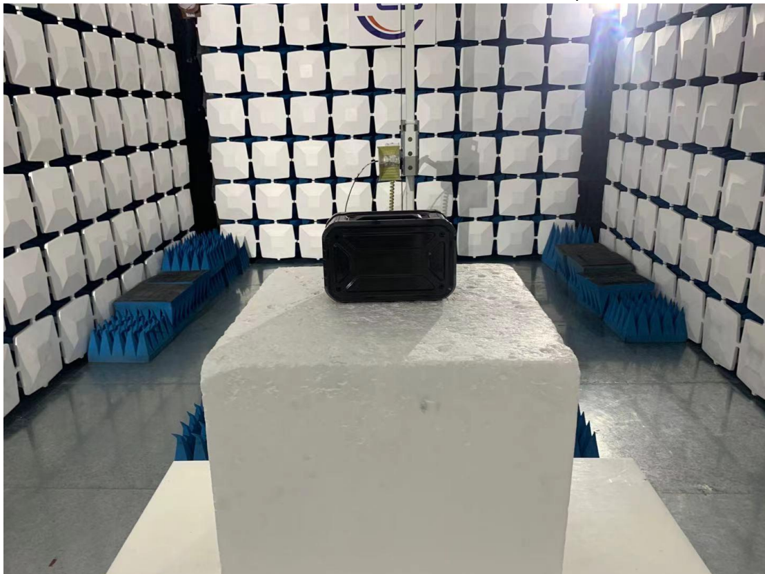
Above 1GHz for radiated emission test setup
