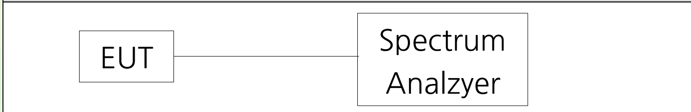
Test Setup for Conducted test
