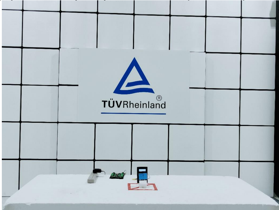
Photograph 1: Test Setup for Spurious Emissions (Front View 1)
