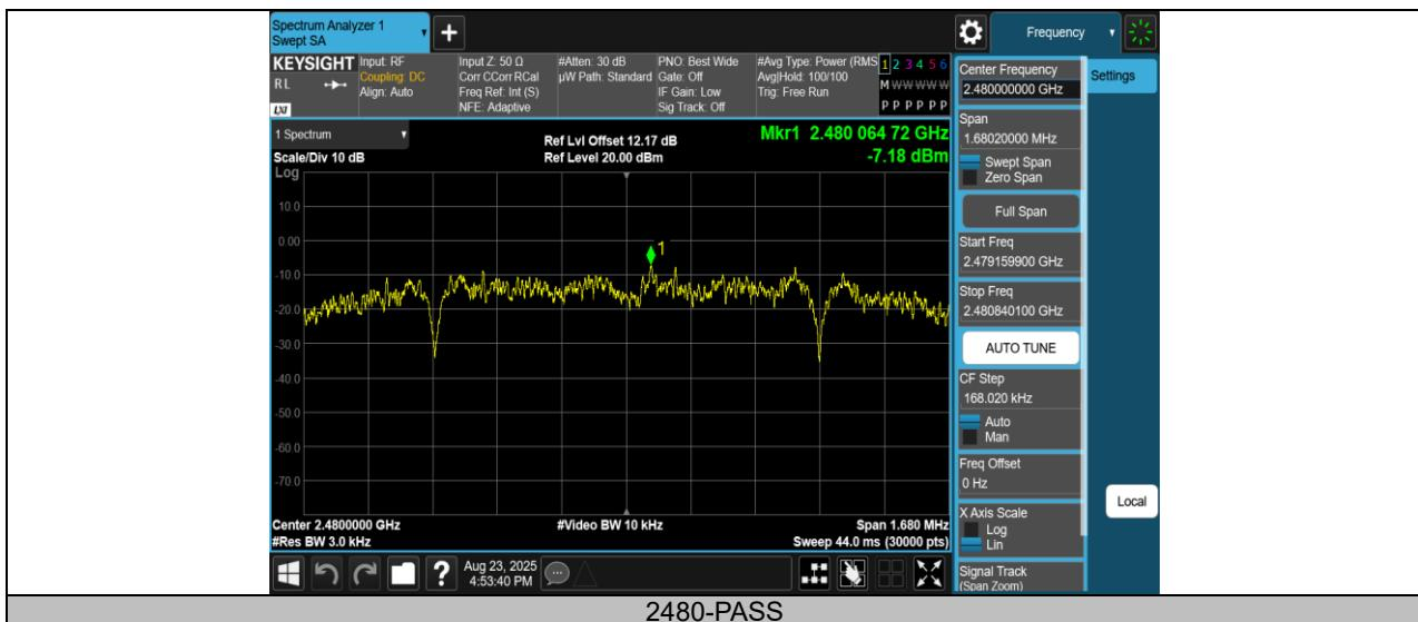
**TEST REPORT****Conducted Spurious Emission****Test Result**
