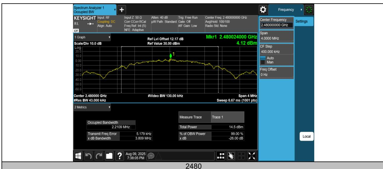
**TEST REPORT****Maximum conducted output power****Test Result Peak**
