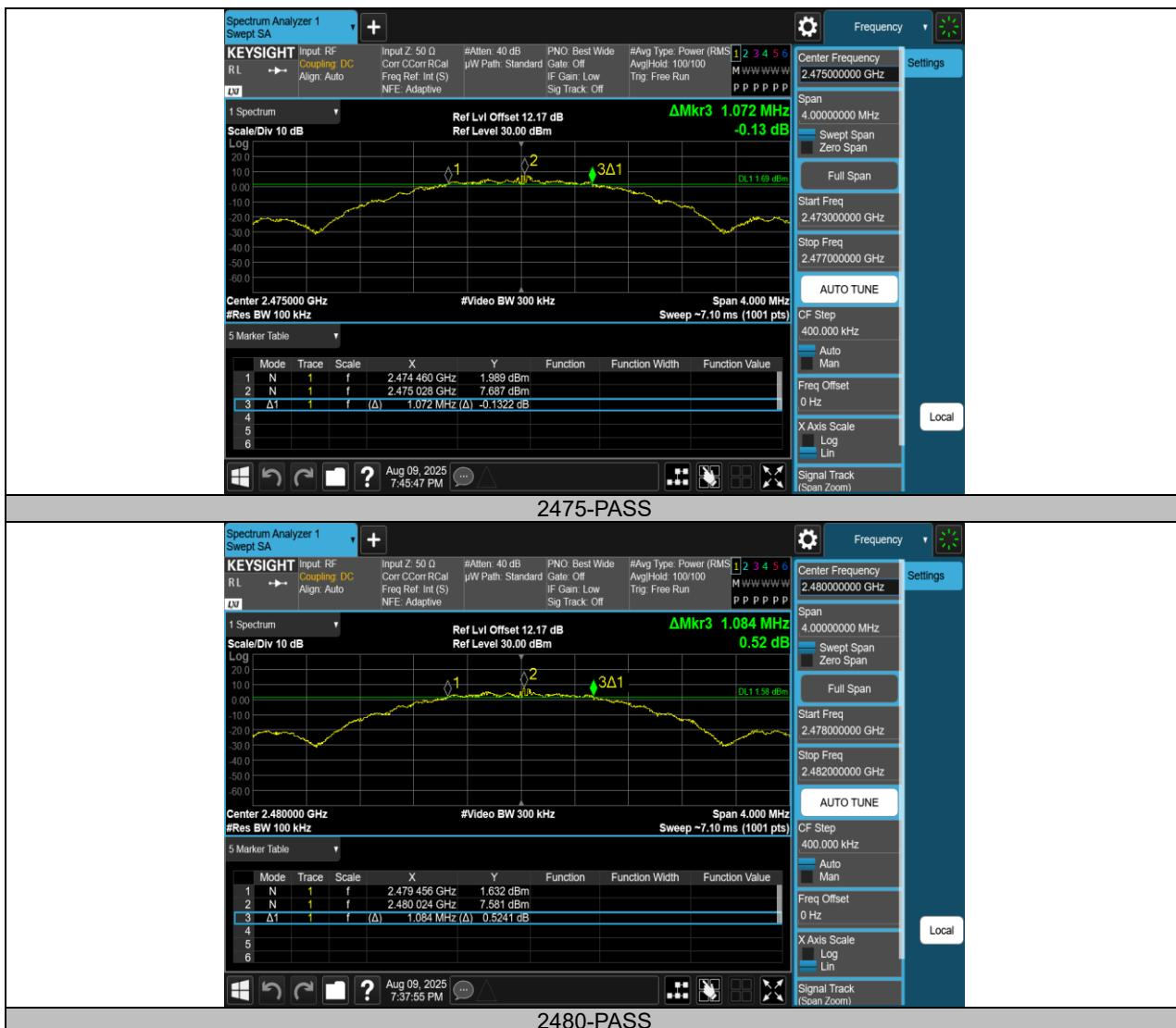
**TEST REPORT****Occupied Channel Bandwidth****Test Result**
