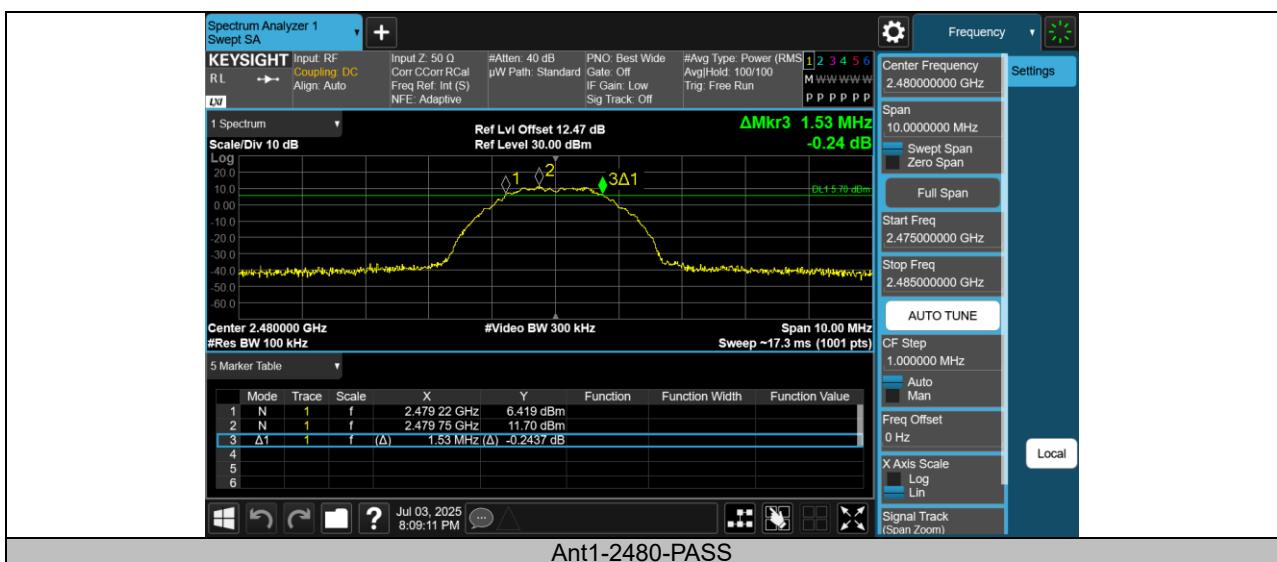
**TEST REPORT****Occupied Channel Bandwidth****Test Result**
