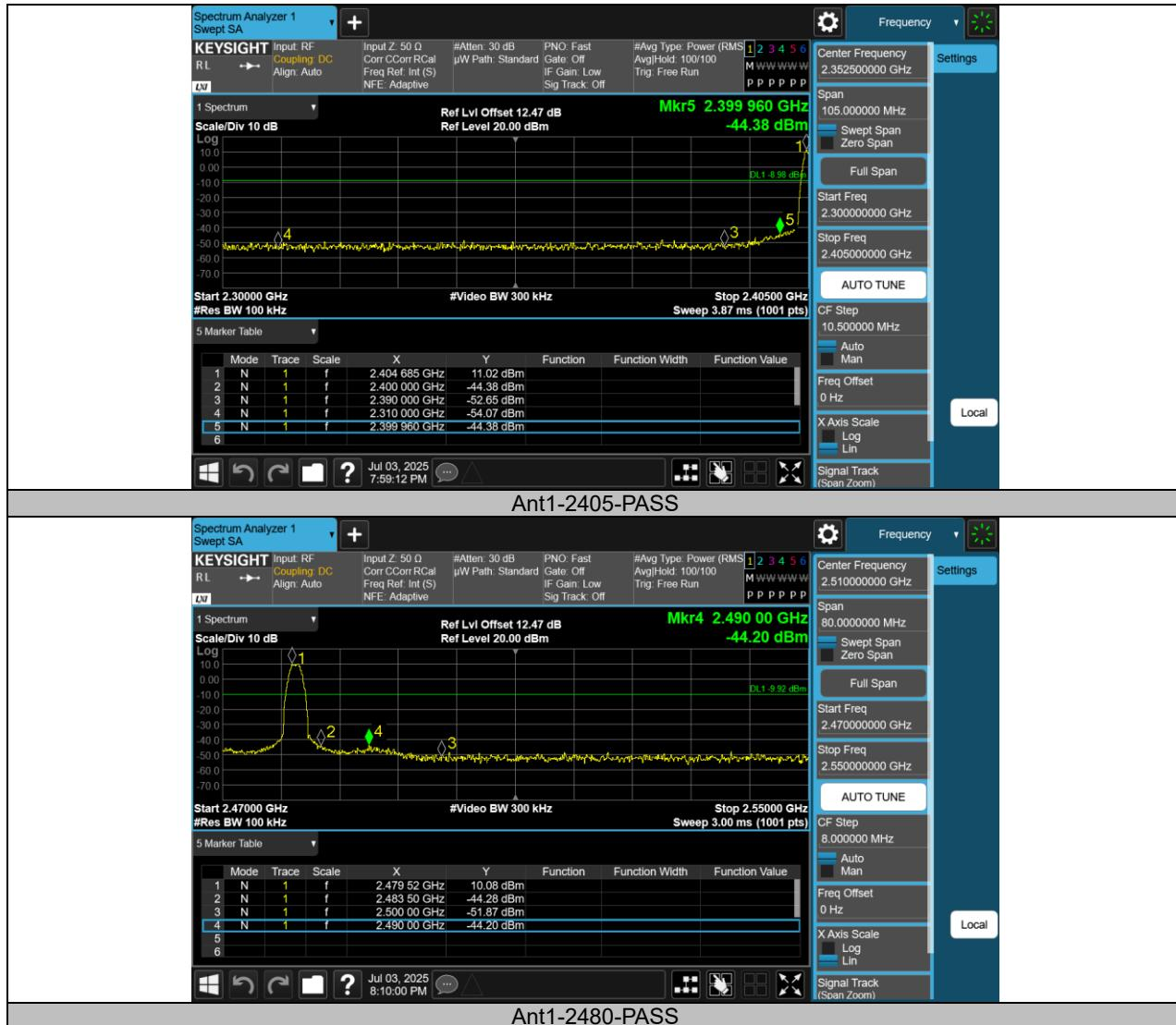
**TEST REPORT****Conducted Spurious Emission****Test Result**
