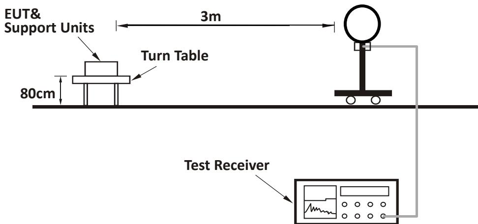
For Radiated emission 30MHz to 1GHz:
