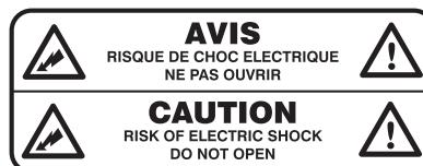
The symbol is used to indicate that some hazardous live terminals are involved within this apparatus, even under the normal operating conditions, which may be sufficient to constitute the risk of electric shock or death.
