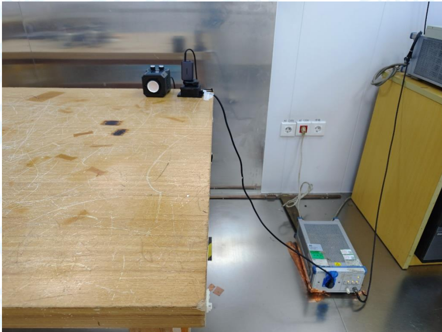
Photo of Setup for Radiated Emission (30MHz~1GHz)
