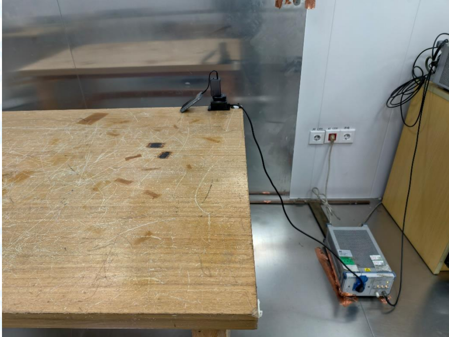
Photo of Setup for Radiated Emission (30MHz~1GHz)
