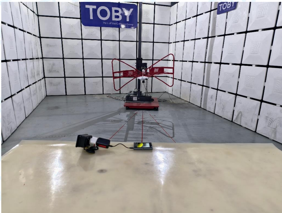
Photo of Setup for Radiated Emission (30MHz~1GHz)
