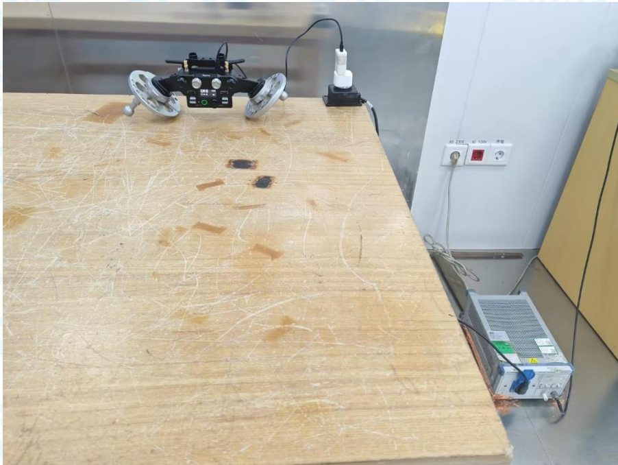
Photo of Setup for Radiated Emission (30MHz~1GHz)
