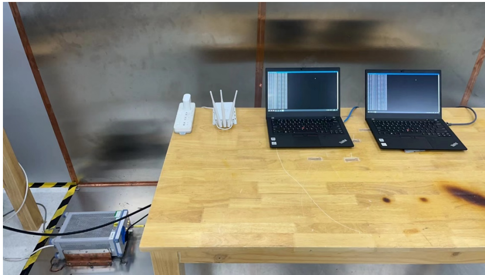
Photograph 3: Set-up photo for Conducted Emission on AC Mains
