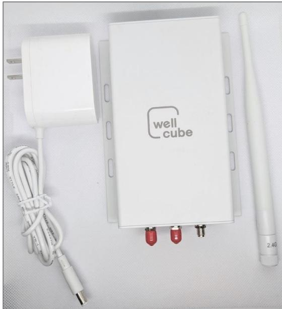
2. Connect one of the supplied 2.4GHz antennas to the Thread antenna connector on the back of the WellCube Connect main body.
