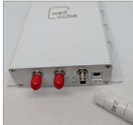
NOTE: WellCube Connect should be placed within 50 ft from the closest WellCube device. Orient the Thread antenna vertically for maximum coverage.
