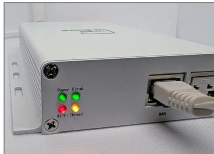
The 4 LED status indicators on the front of WellCube connect will display different colors to indicate various connectivity states or errors as shown below. Once commissioned, the Cloud LED will display solid green, indicating that other WellCube devices can now be commissioned to the Thread network.
