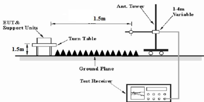
The radiated emission tests were performed in the 3 meters chamber test site, using the setup accordance with the ANSI C63.10-2013. The specification used was FCC 15.209, FCC 15.407 limits.
