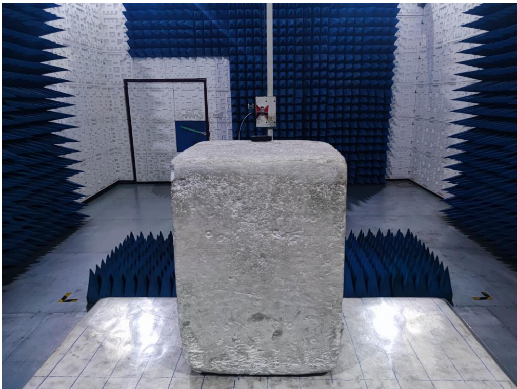
RADIATED EMISSION TEST SETUP ABOVE 1GHz
