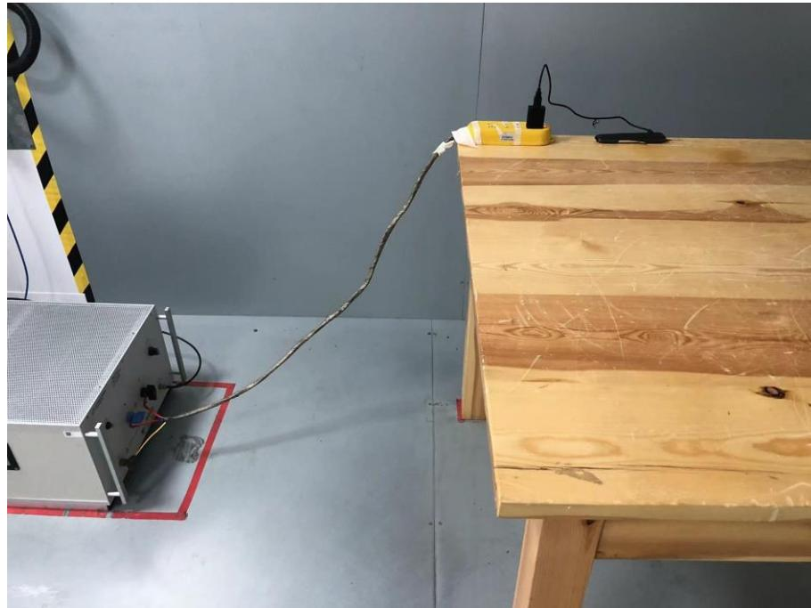
**Set-up for Radiated Emission (RE), Below 1GHz**
