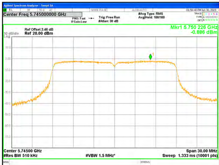
PSD NVNT n20 5745MHz Ant1
