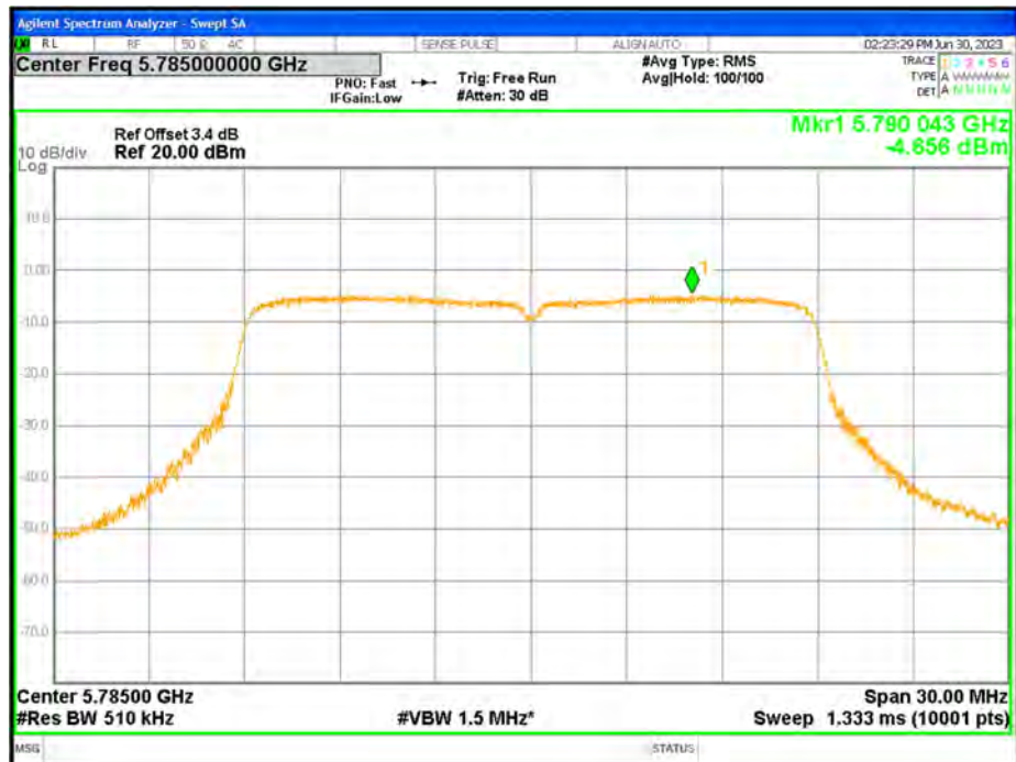
PSD NVNT ac20 5785MHz Ant1
