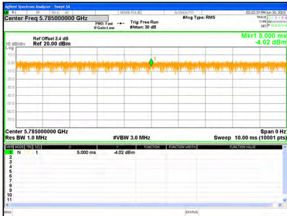
Duty Cycle NVNT ac20 5785MHz Ant1
