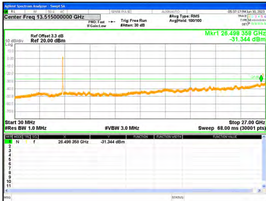
Tx. Spurious NVNT n40 5190MHz Ant1 Emission
