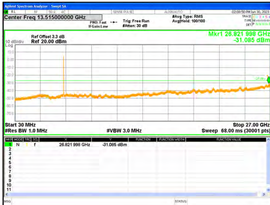
Tx. Spurious NVNT ac20 5180MHz Ant1 Emission
