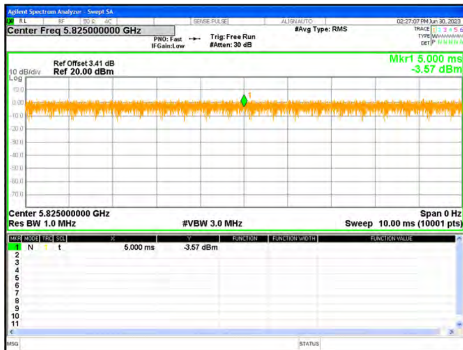
Duty Cycle NVNT ac20 5825MHz Ant1
