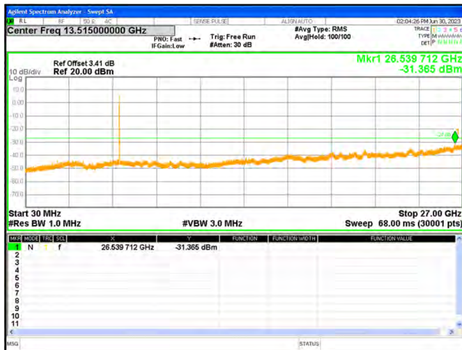
Tx. Spurious NVNT n20 5825MHz Ant1 Emission
