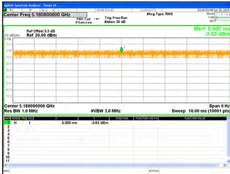
Duty Cycle NVNT ac20 5180MHz Ant1
