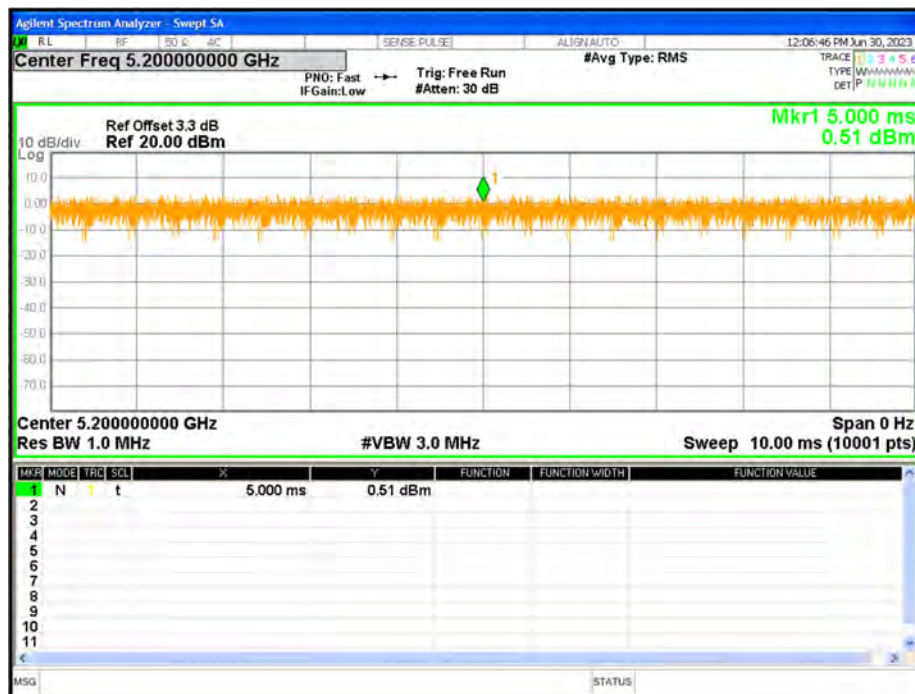
Duty Cycle NVNT n20 5200MHz Ant1
