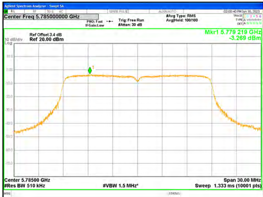
PSD NVNT n20 5785MHz Ant1
