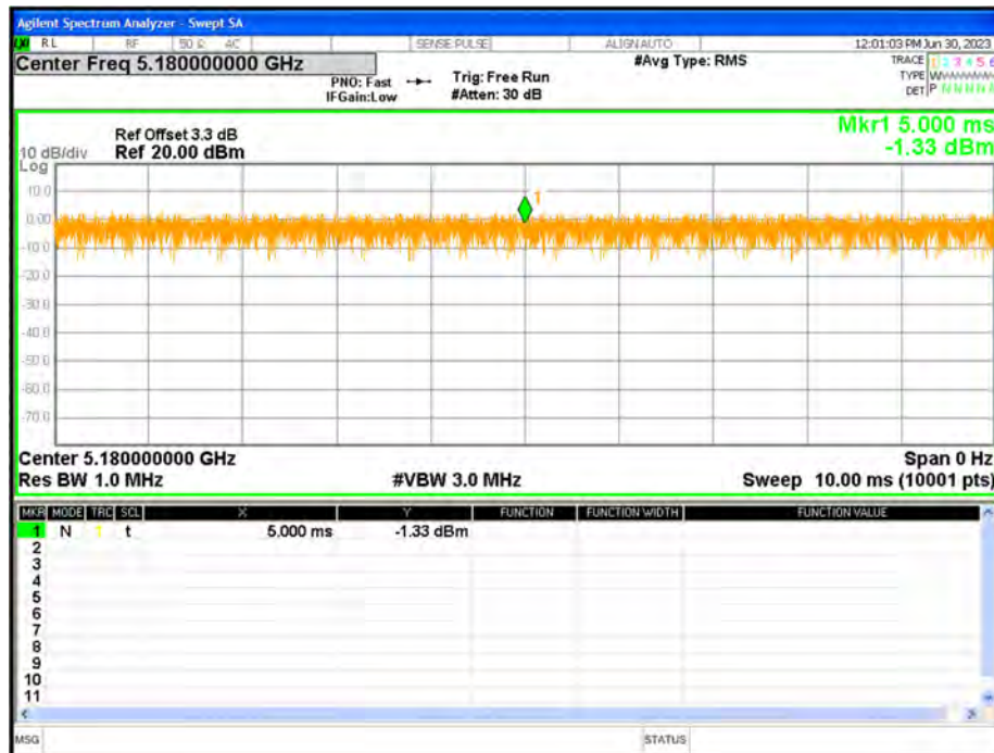
Duty Cycle NVNT n20 5180MHz Ant1
