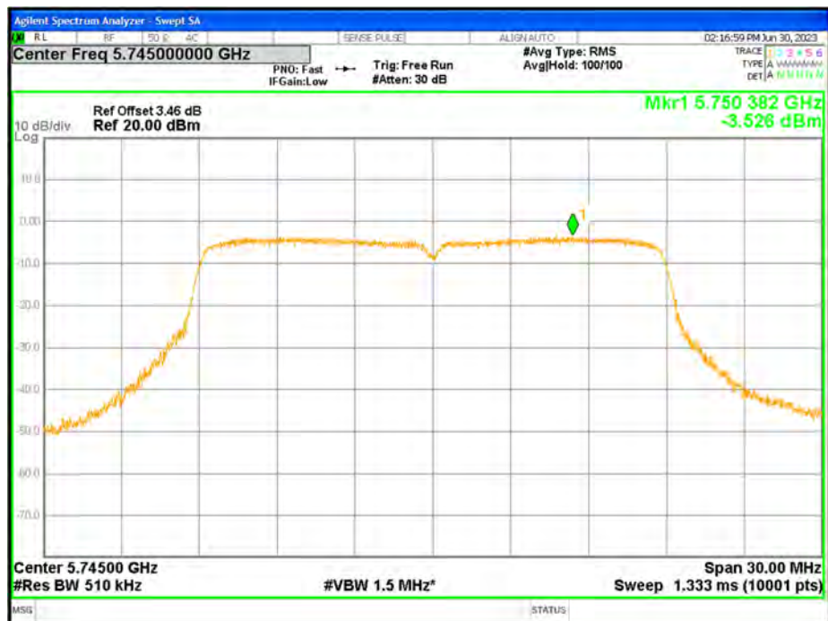
PSD NVNT ac20 5745MHz Ant1
