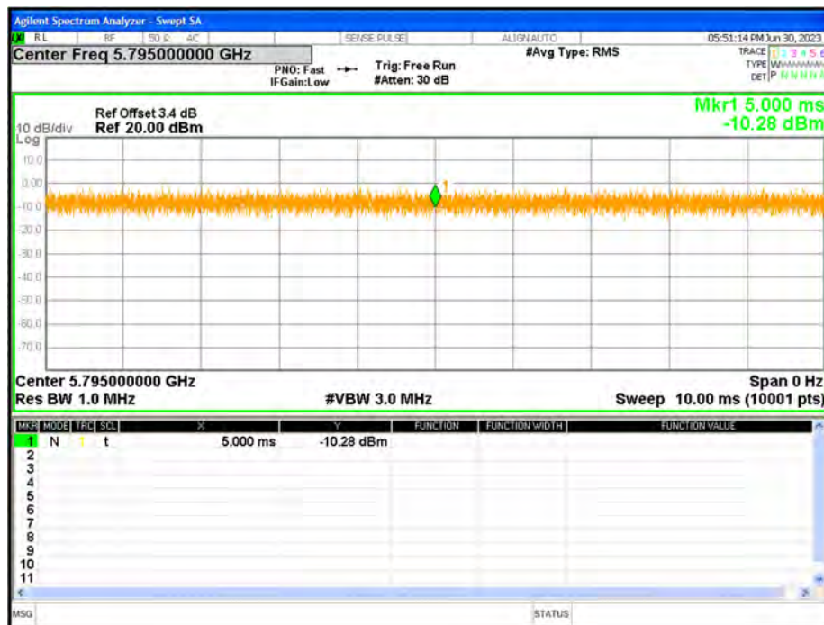
Duty Cycle NVNT n40 5795MHz Ant1
