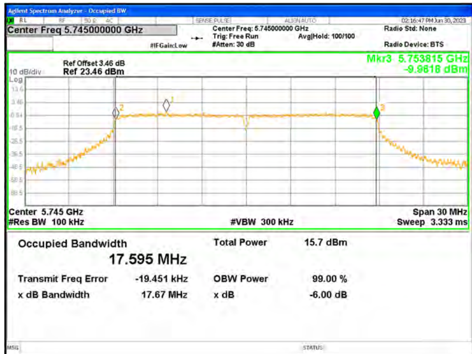
-6dB Bandwidth NVNT ac20 5745MHz Ant1
