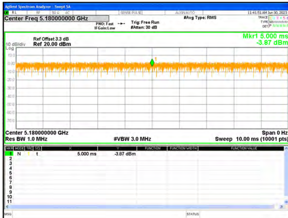
Duty Cycle NVNT a 5180MHz Ant1
