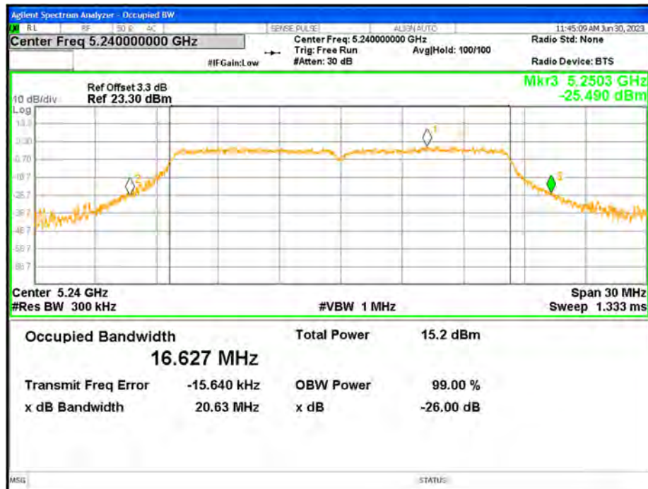
-26dB Bandwidth NVNT a 5240MHz Ant1
