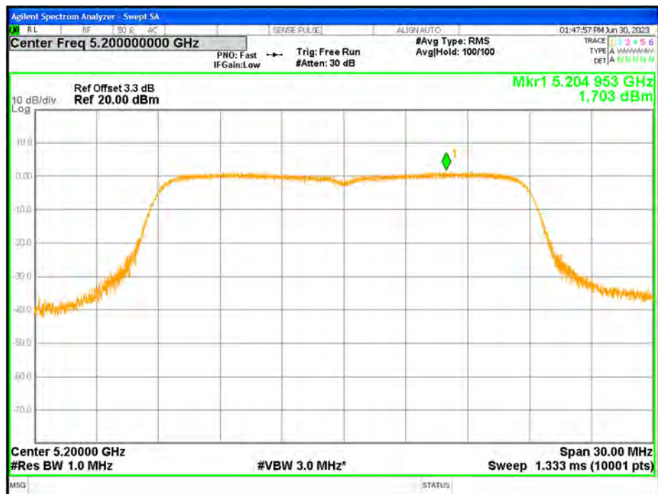
PSD NVNT n20 5200MHz Ant1
