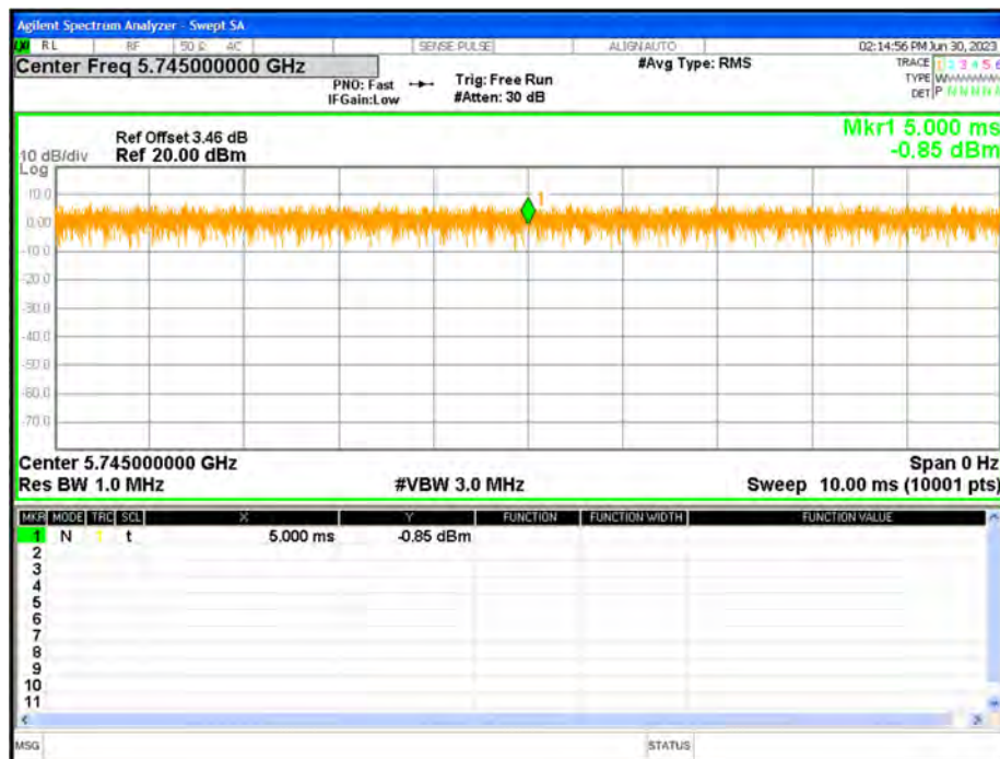
Duty Cycle NVNT ac20 5745MHz Ant1
