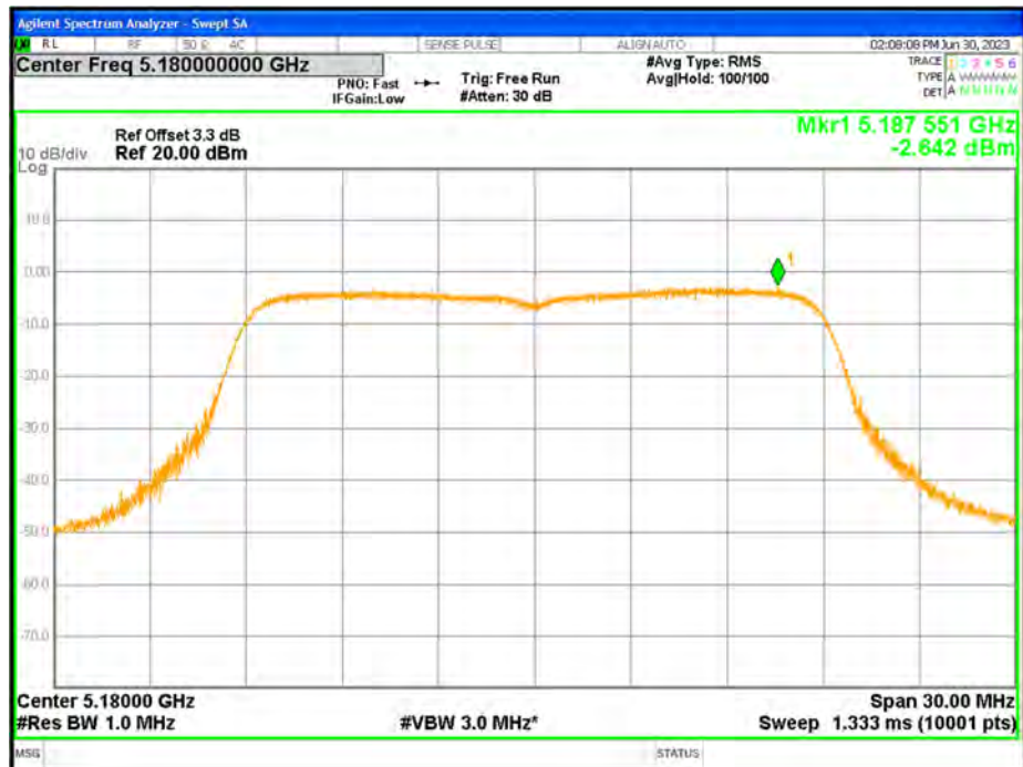
PSD NVNT ac20 5180MHz Ant1
