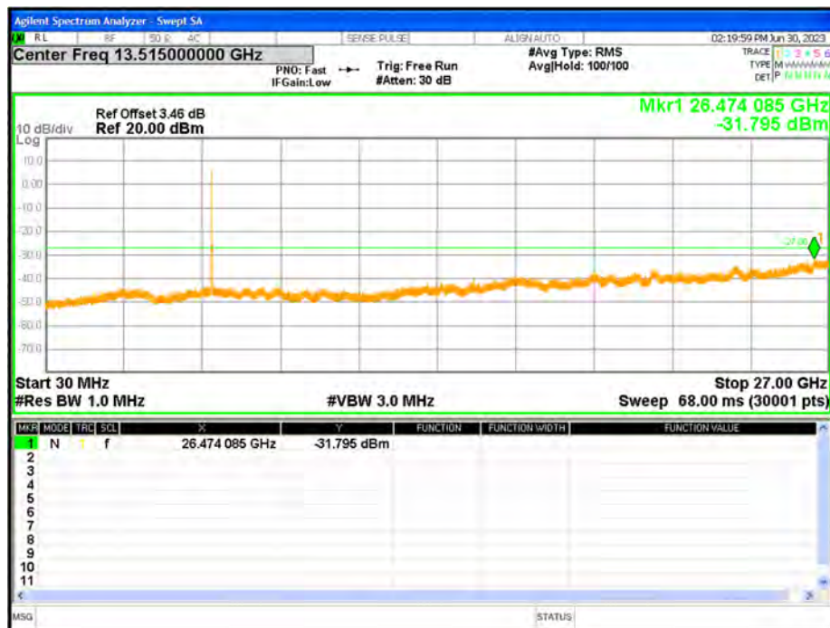
Tx. Spurious NVNT ac20 5745MHz Ant1 Emission
