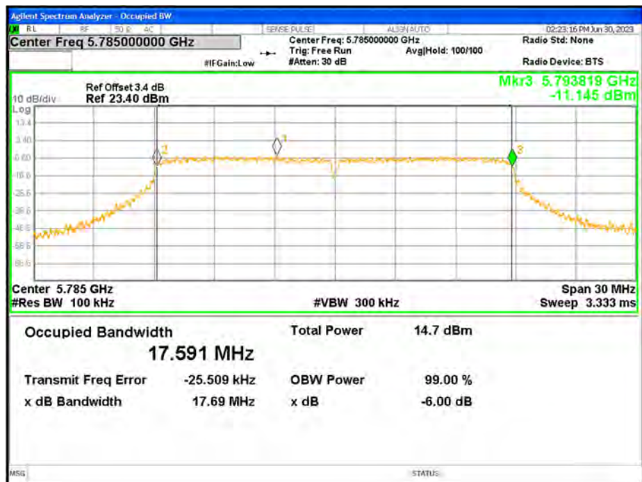
-6dB Bandwidth NVNT ac20 5785MHz Ant1
