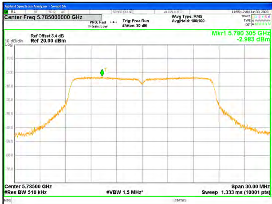
PSD NVNT a 5785MHz Ant1
