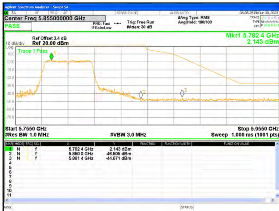
Band Edge NVNT ac40 5795MHz High Ant1
