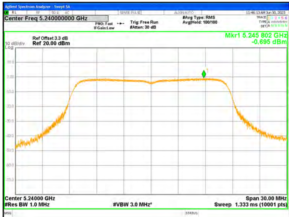
PSD NVNT a 5240MHz Ant1
