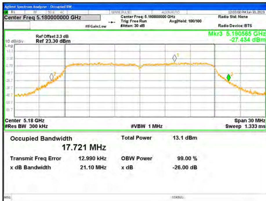
-26dB Bandwidth NVNT n20 5180MHz Ant1
