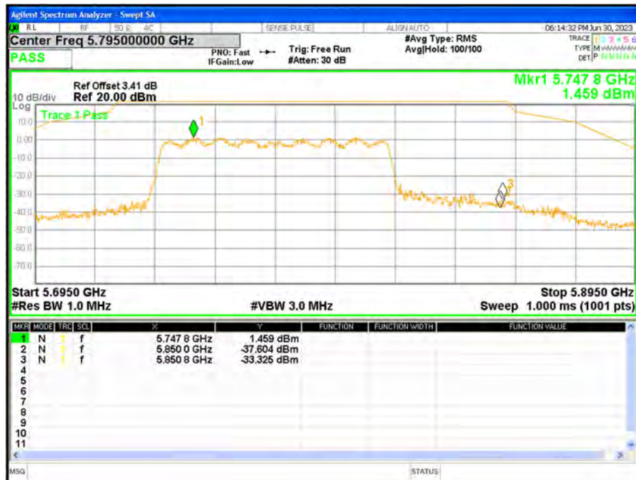
Band Edge NVNT ac80 5775MHz High Ant1
