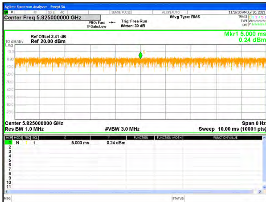
Duty Cycle NVNT a 5825MHz Ant1
