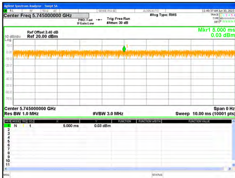
Duty Cycle NVNT a 5745MHz Ant1
