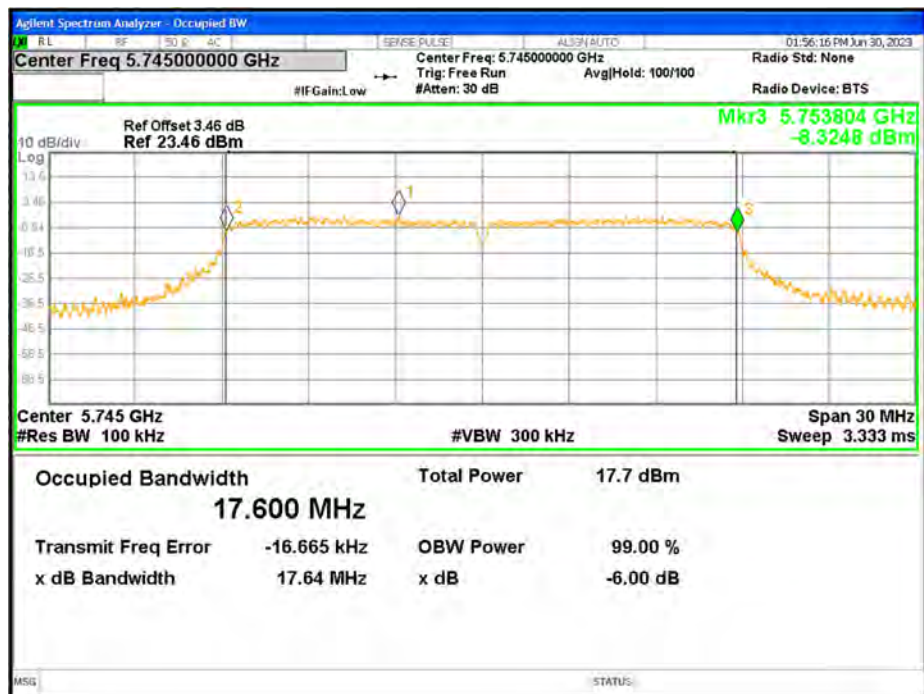
-6dB Bandwidth NVNT n20 5745MHz Ant1
