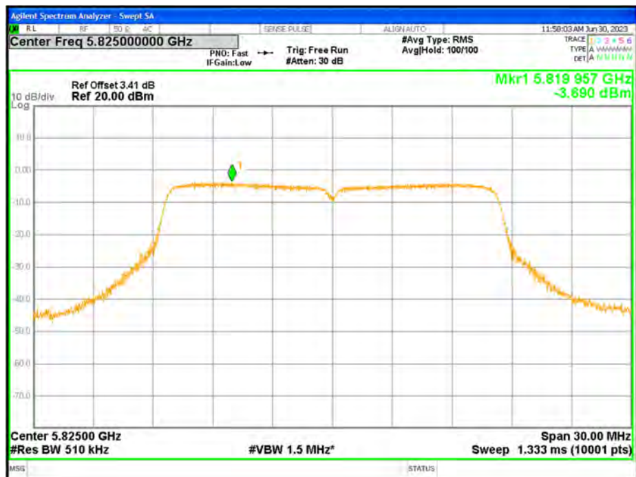
PSD NVNT a 5825MHz Ant1
