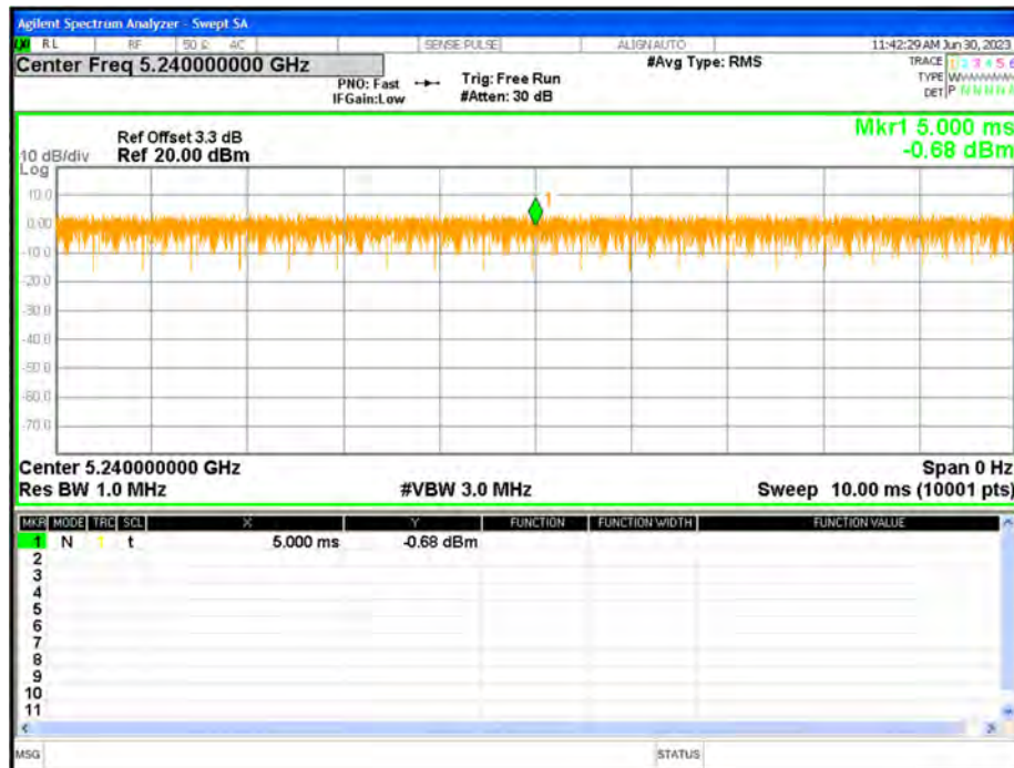
Duty Cycle NVNT a 5240MHz Ant1
