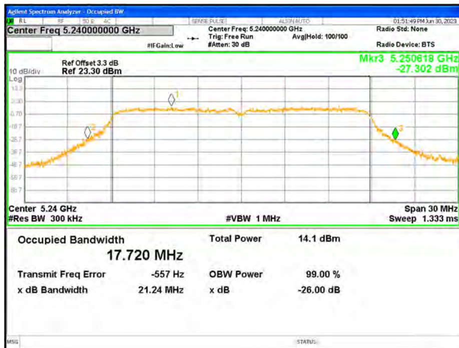
-26dB Bandwidth NVNT n20 5240MHz Ant1
