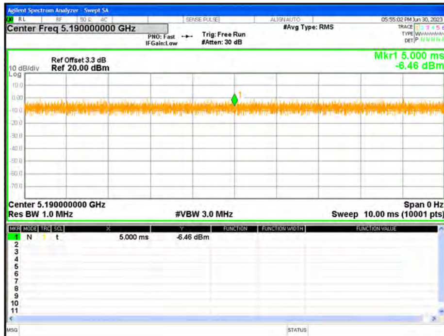
Duty Cycle NVNT ac40 5190MHz Ant1
