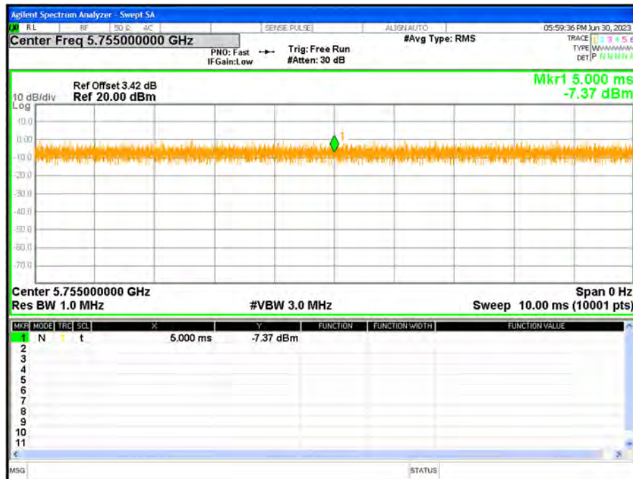
Duty Cycle NVNT ac40 5755MHz Ant1
