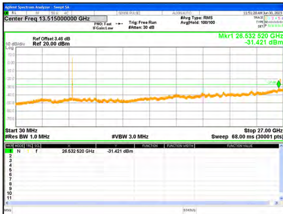
Tx. Spurious NVNT a 5745MHz Ant1 Emission
