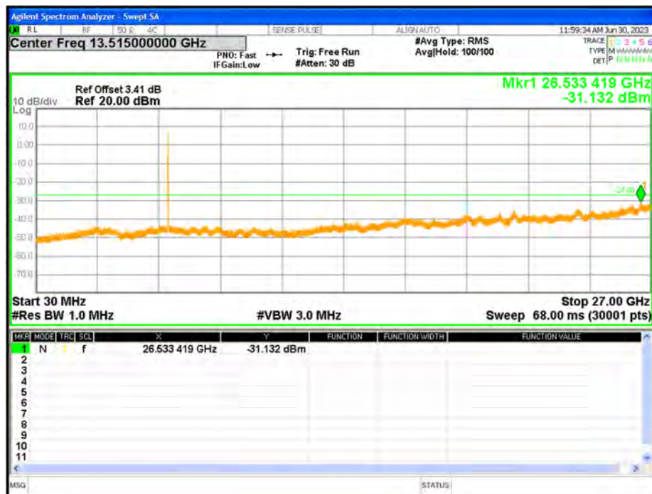
Tx. Spurious NVNT a 5825MHz Ant1 Emission
