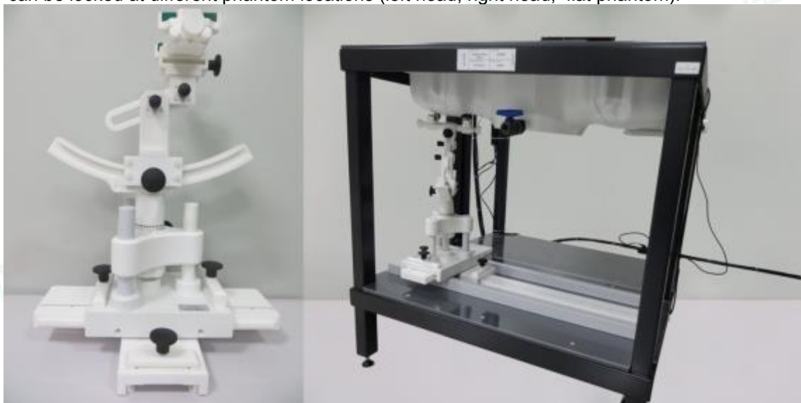
Device holder supplied by SATIMO
