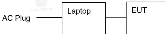
Operation of EUT during radiation above 1GHz testing:
