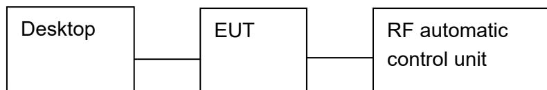
The sample was placed (0.8m below 1GHz, 1.5m above 1GHz) above the ground plane of 3m chamber. Measurements in both horizontal and vertical polarities were performed.
