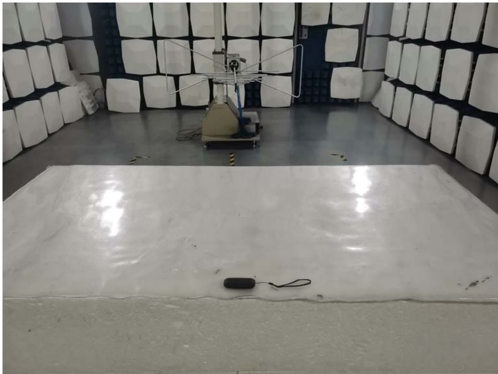
Radiated emission test view:
