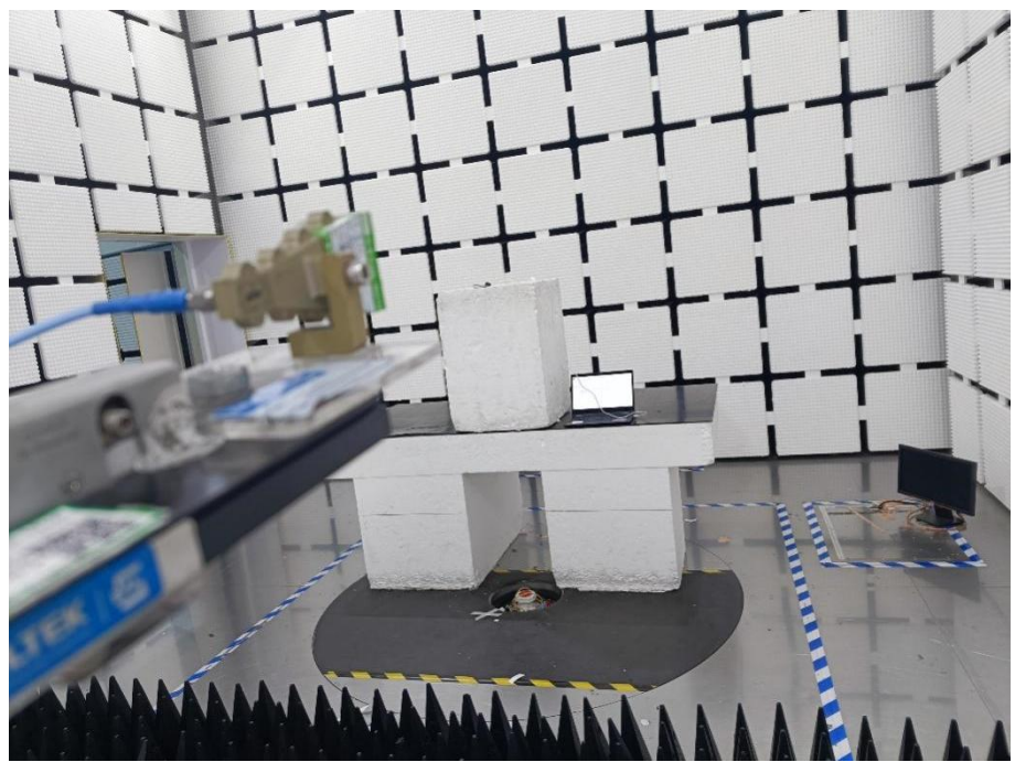
Radiation Emission Test Setup (Above 18GHz)
