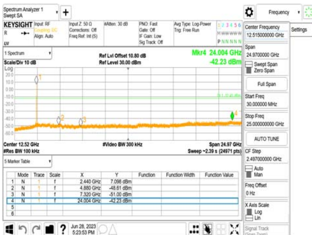
Spurious Emission_BLE 2M_MidCH19-2440MHz
