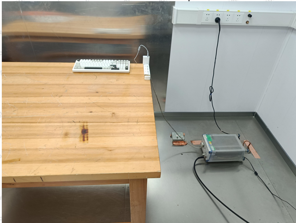
Photo of Radiation Emission Test (below 1GHz)
