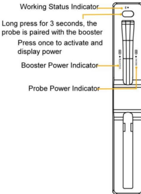
The probe can be used for more than 24 hours after full charge.
