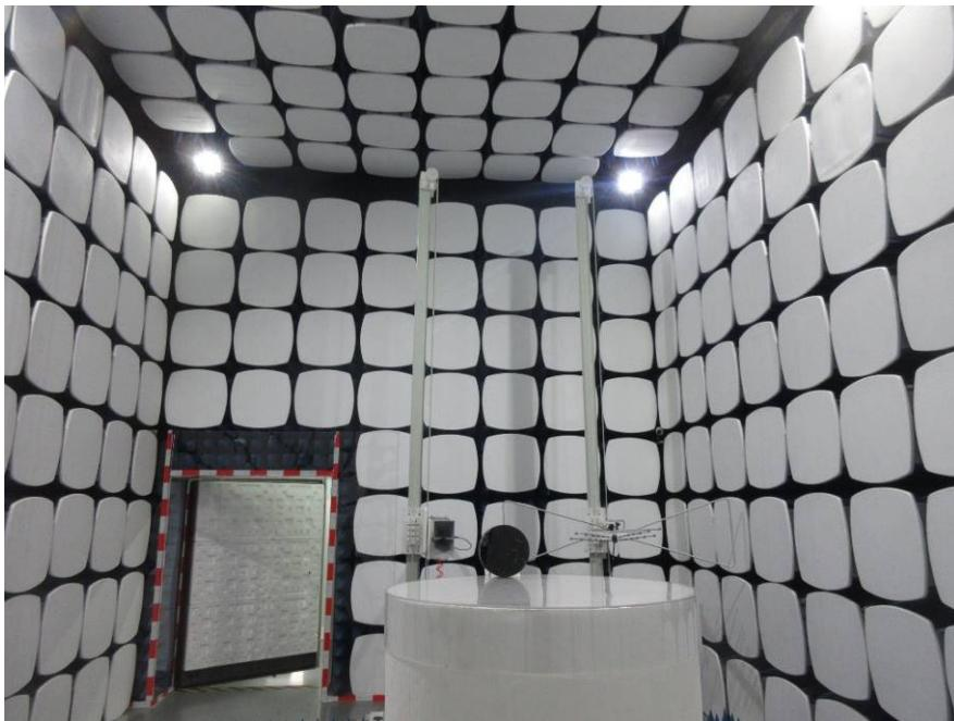
**Radiated Emissions which fall in the restricted bands & Radiated Spurious Emissions Below 1GHz**
